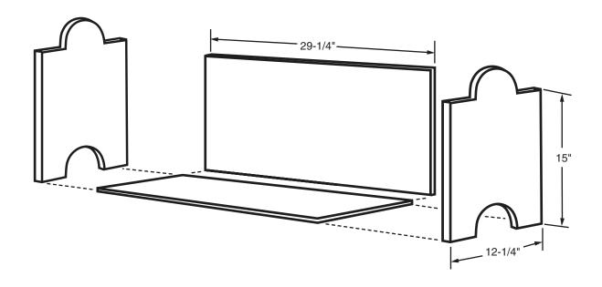
NOTE: ENDS ARE GLUED AND DOWELED WITH 1/4" x 1-1/2" DOWELS TO SHELVES AND BACKS
